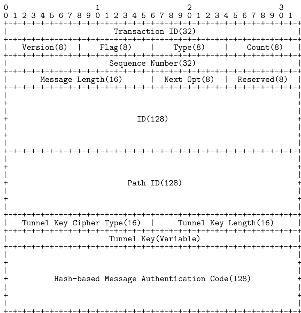
図 A.12 Structure of Relay Response
